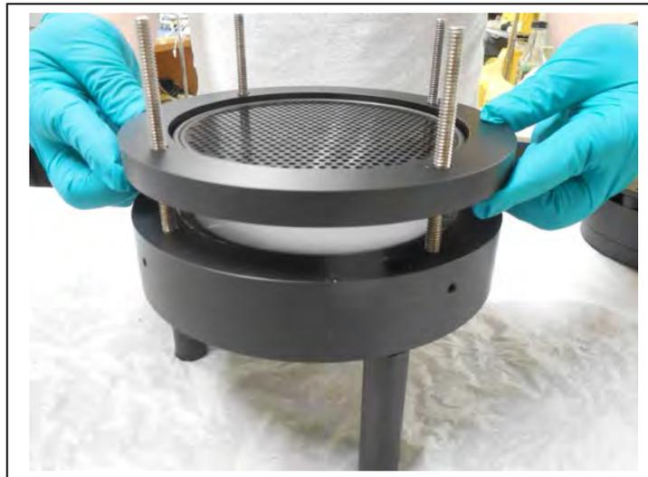
*Figure 6.1-6: Placing the Pre-Filter Plate on the Filter Holder*
