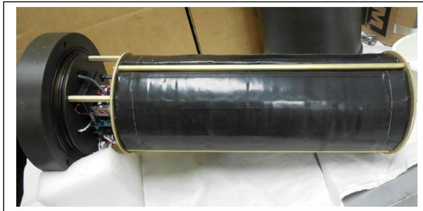
*Figure C.2-2: WTS-LVUP Controller with A72-1000 Battery Pack*
