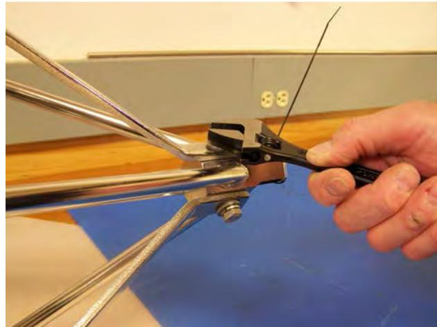
*Figure C.3-8: Loosening Frame Guard*
