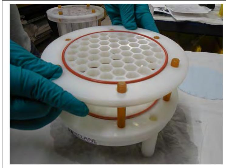
*Figure 6.2-4: Installing the Pre-Filter Plate*
