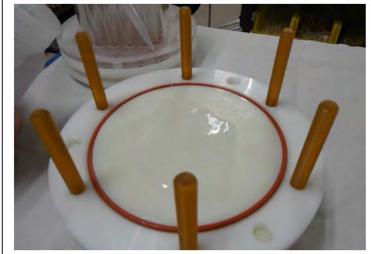
*Figure 6.2-2: Flood the Filter Holder Bottom Plate*
