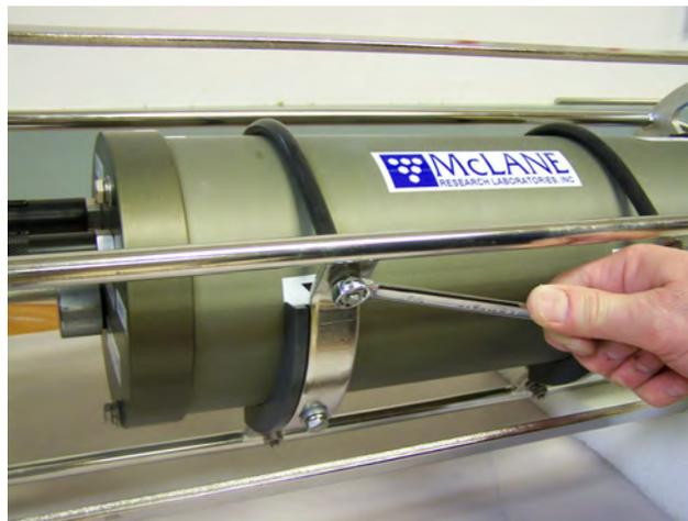
*Figure C.3-10: Loosening U-Bolt Clamp*
