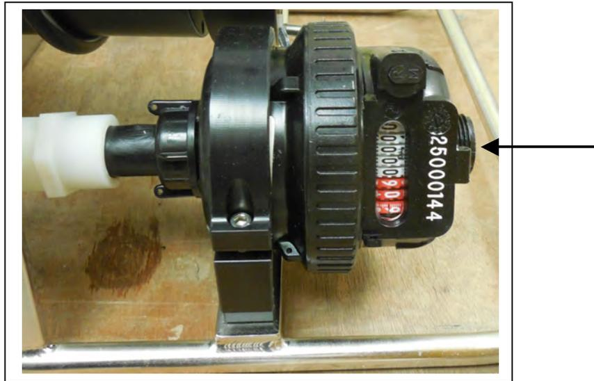
*Figure D-4: Exhaust Port*
