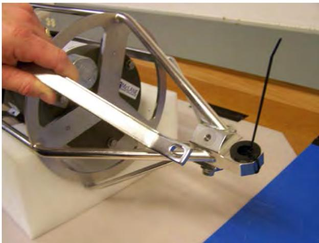
*Figure C.3-9: Removing Leg Bolt*
