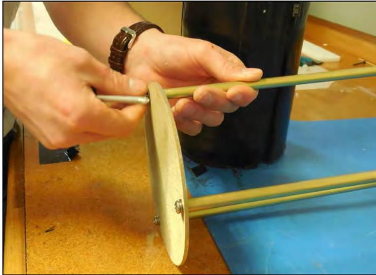
*Figure C.2-3: Removing Battery Housing End Plate*
