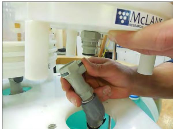
*Figure C.1.2-4: Lifting Filter Holder off of Plate*
