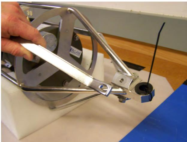
*Figure C.3-9: Removing Leg Bolt*
