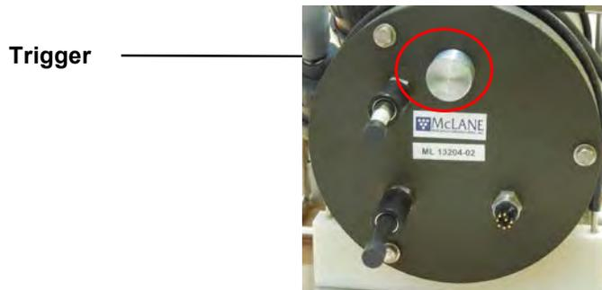
*Figure 3-24: Trigger Plug*
