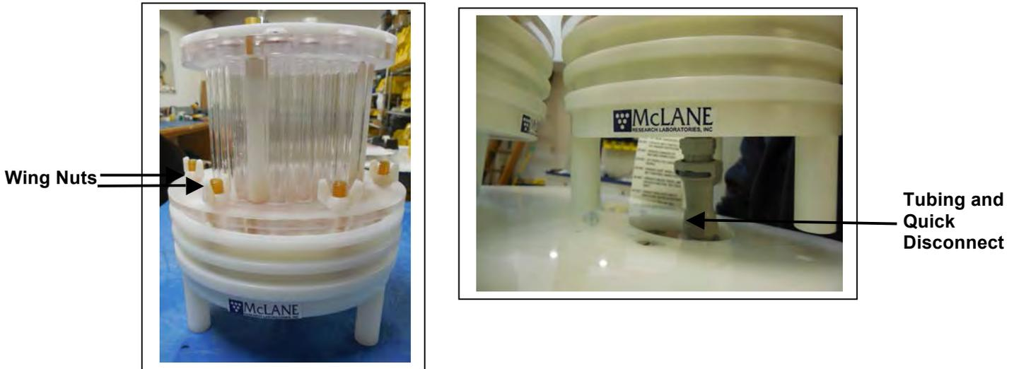
*Figure 6.2-1: Vertical Intake Filter Holder*
