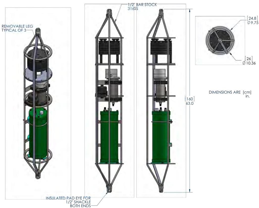
Figure C.3-2: Bore-Hole WTS-LV Schematic
