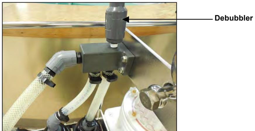
*Figure C.1.3-2: Screw Debubbler into Manifold*
