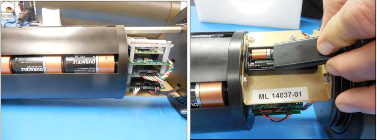
*Figure C.3-13: Main and Backup Batteries*
