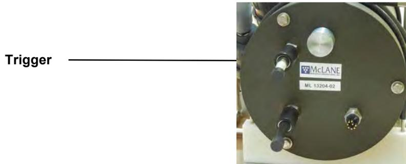
*Figure 5-6: Trigger Plug*
