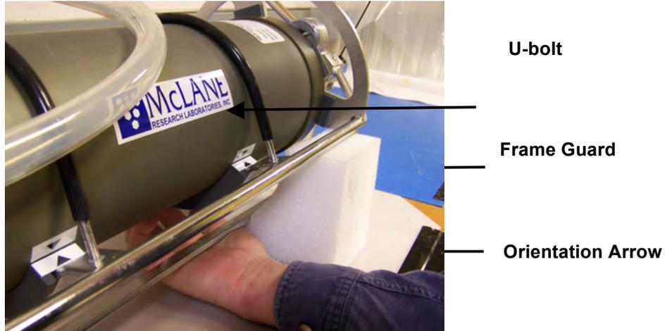
*Figure C.3-3: WTS-LV Frame Guards, U-Bolts and Orientation Arrows*
