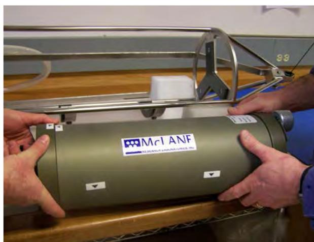
*Figure C.3-12: Removing Controller Housing*
