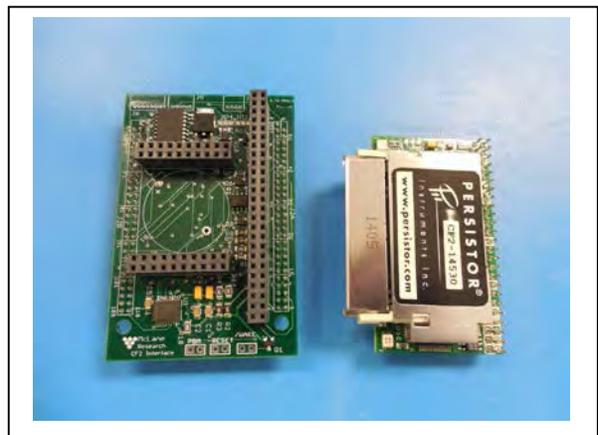
Figure 5-2: Microcontroller & Interface Board
