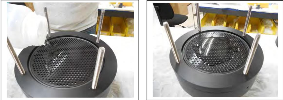
*Figure 6.1-7: Fill the Pre-Filter Plate until Water Pools*
