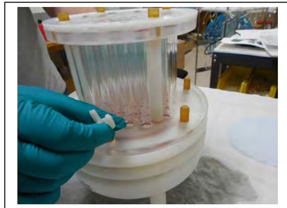
*Figure 6.2-8: Install Filter Top and Tighten Wing Nuts*
