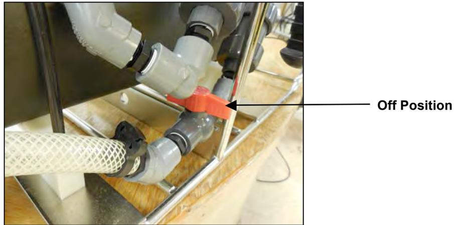
*Figure C.1.3-10: Setting the Flow Valve*
