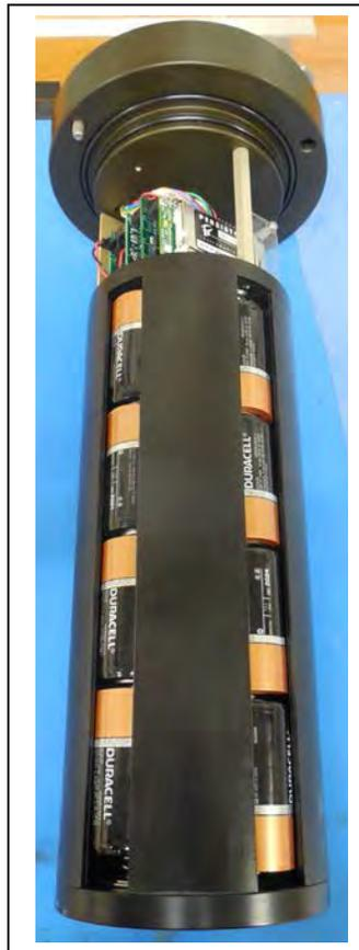
*Figure 8-2: Battery Orientation in Holder*
