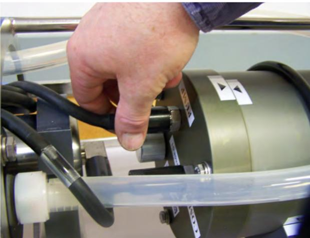
*Figure C.3-7: Removing Connector*
