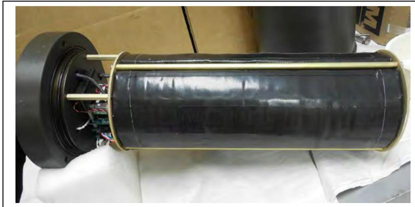
*Figure C.1.3-3: WTS-LVDF Controller with A72-1000 Battery Pack*
