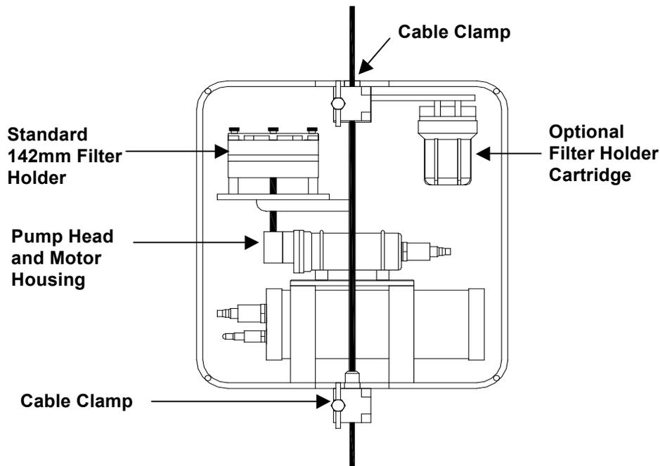
*Figure 1-2: WTS-LV Line Drawing - Side View*
