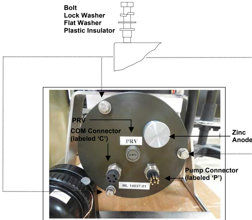
*Figure 4-6: Controller Housing End Cap Bulkhead Connectors*
