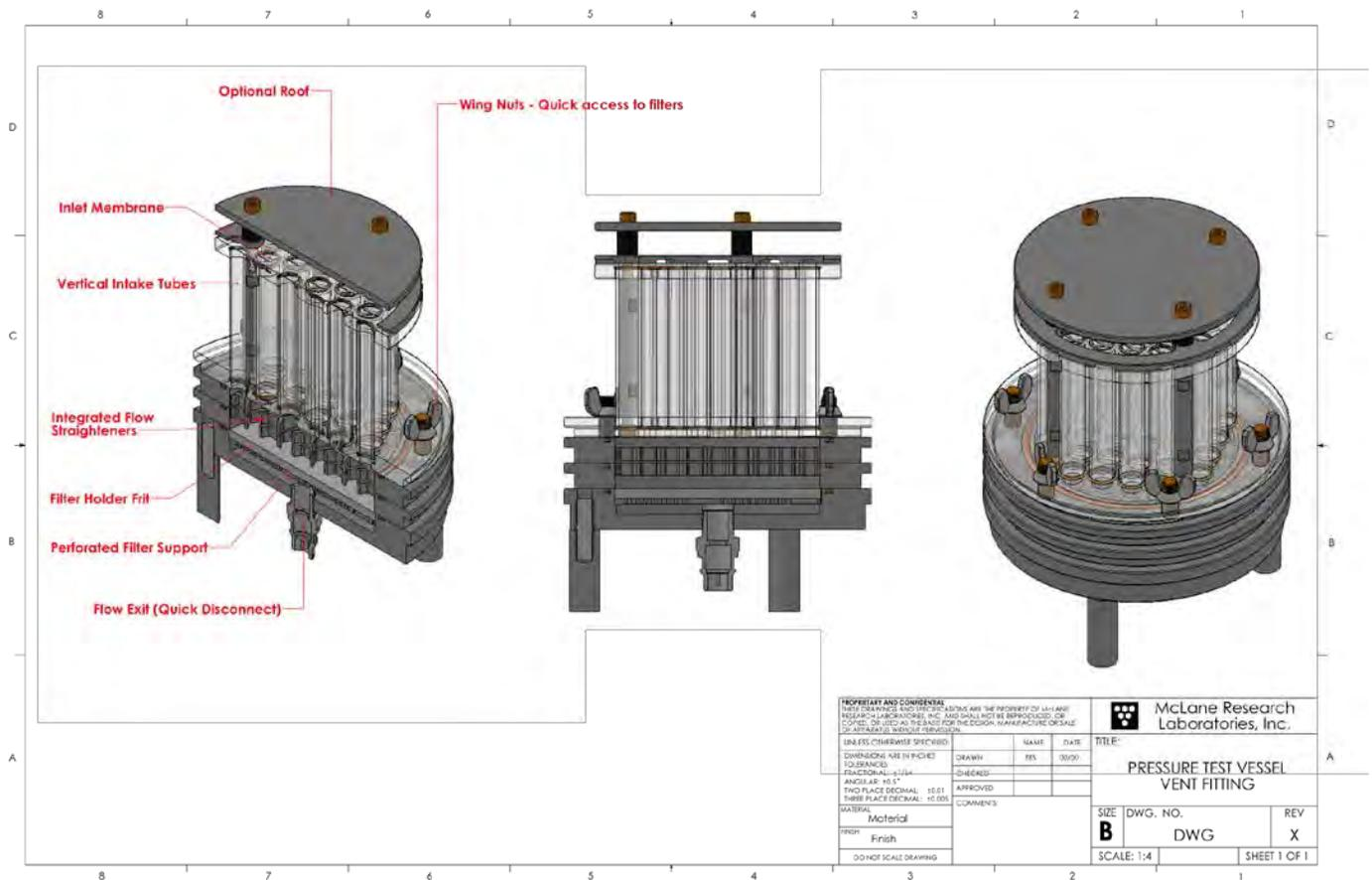
Figure C.1.1-1: WTS-LVDF Filter Holder Cross Section
