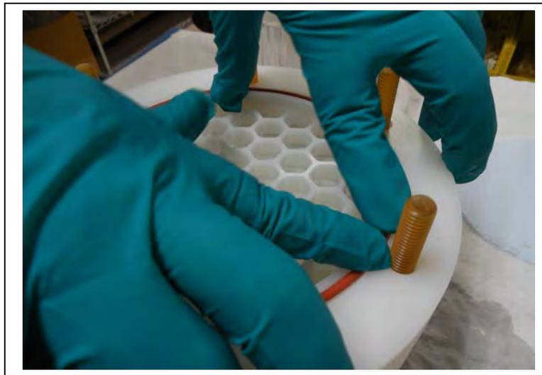
*Figure 6.2-5: Secure Seal in Plate Groove*
