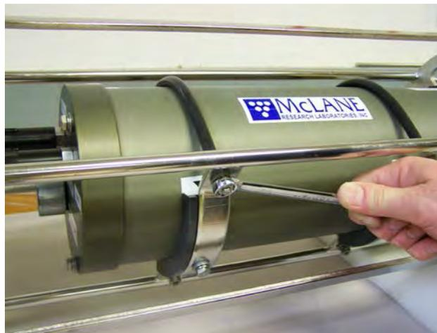
*Figure C.3-10: Loosening U-Bolt Clamp*
