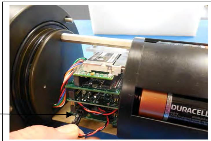
*Figure 2-9: Connecting Main Battery to the Electronics Stack*
