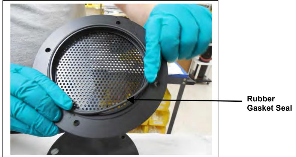
*Figure 6.1-5: Seating the Pre-Filter Plate Rubber Gasket*
