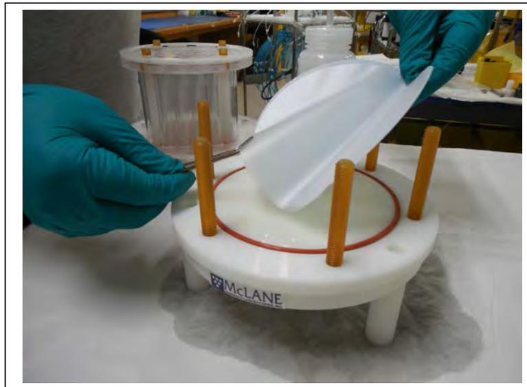
*Figure 6.2-3: Placing the Filter onto the Filter Holder Plate*
