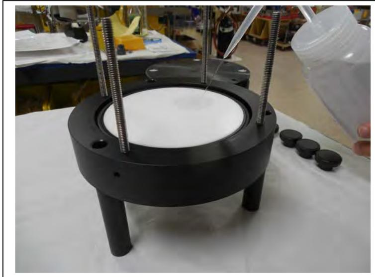
*Figure 6.1-2: Wetting the Bottom Filter Holder Plate*
