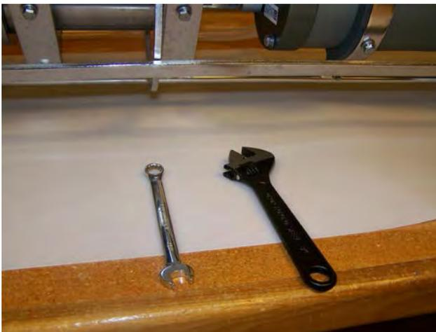
*Figure C.3-4: 7/16" Box Wrench, Adjustable Wrench*
