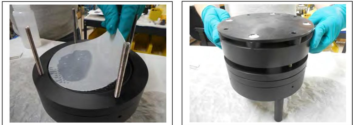
*Figure 6.1-8: Install Filter and Top Section*
