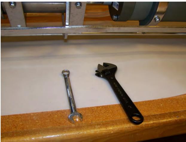
*Figure C.3-4: 7/16" Box Wrench, Adjustable Wrench*
