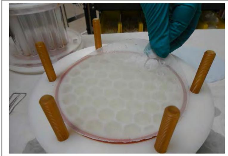
*Figure 6.2-6: Installing the Pre Filter*
