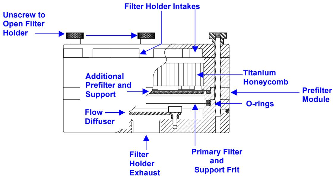
*Figure 4-10: 142mm Standard Filter Holder Schematic*
