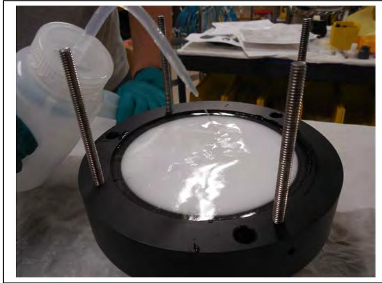
*Figure 6.1-4: Soaking the Installed Filter*
