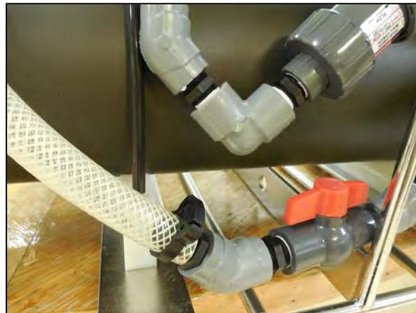
*Figure C.1.2-6: Flow Valve Positioned for Dual Filtering*
