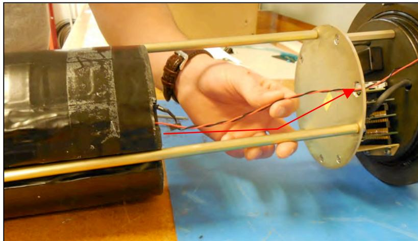
*Figure C.1.3-5: Align Battery to Fit Connector Through Hole in Top Plate*
