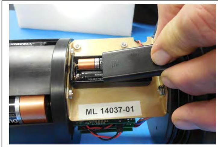
*Figure 2-10: Connecting Main Battery to the Electronics Stack*
