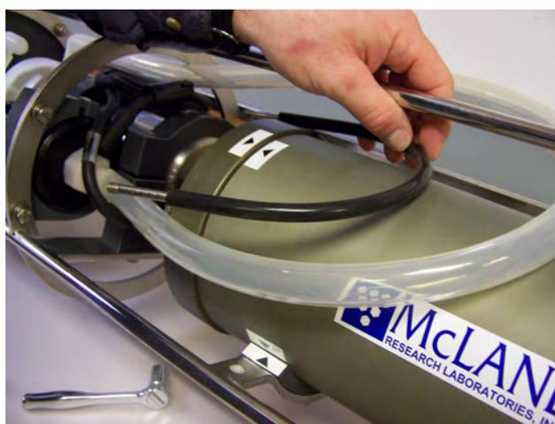
*Figure C.3-11: Removing U-Bolt*
