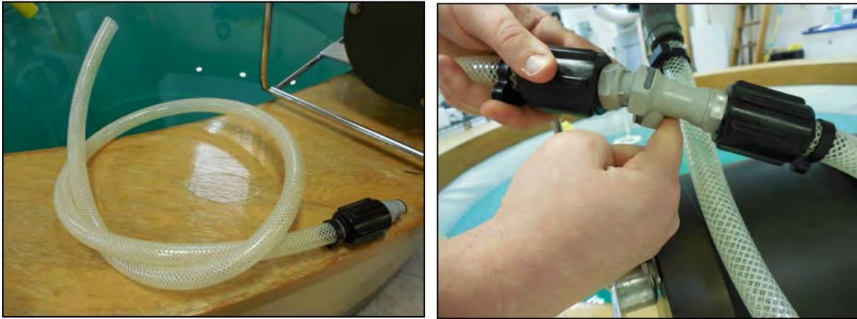
Figure C.1.3-8: Priming Tubing and Quick Disconnect
