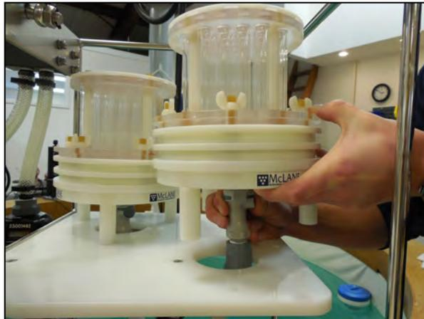
*Figure C.1.2-5: Securing Filter Holder to Quick Disconnect*
