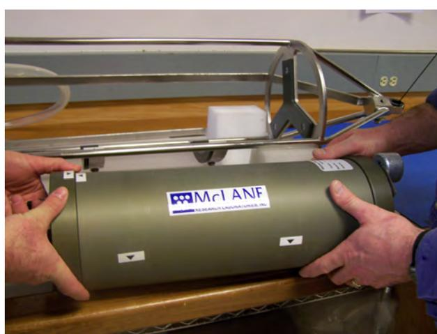
*Figure C.3-12: Removing Controller Housing*
