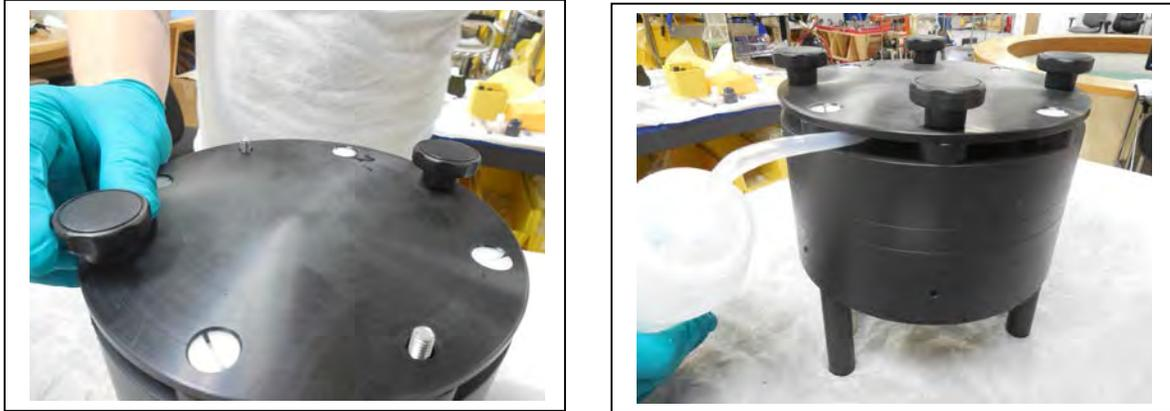
*Figure 6.1-9: Tighten Nuts and Fill Assembly with Neutral Water*
