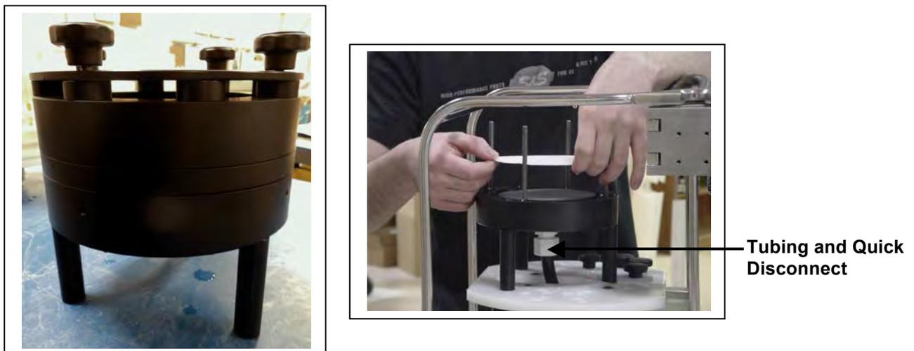
Figure 6.1-1: Standard Filter Holder
