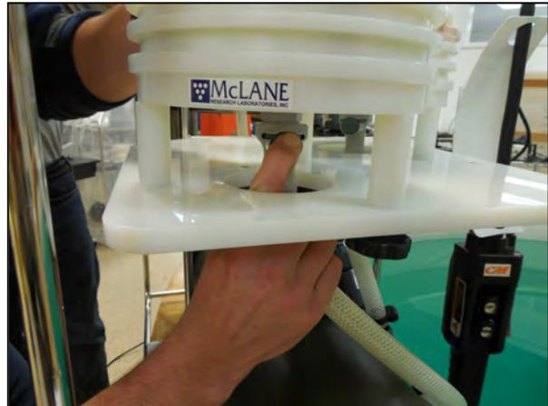
*Figure C.1.2-3: Remove Nuts and Release Quick Disconnect*
