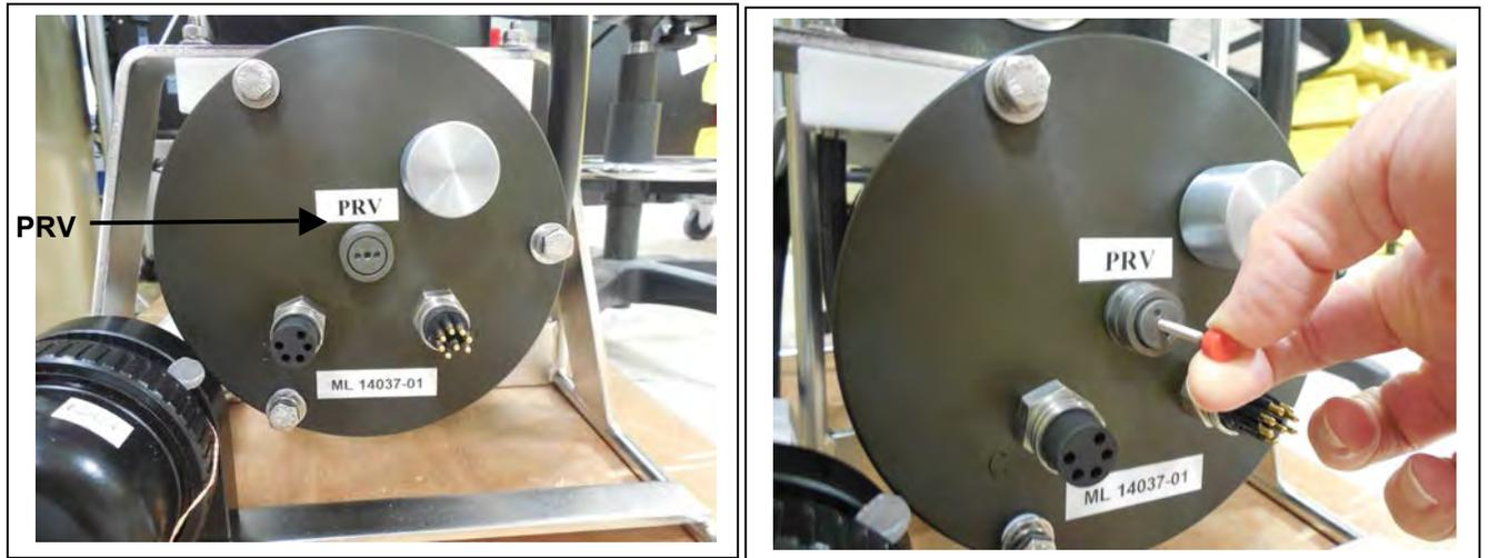
*Figure 4-7: Controller End Cap, with PRV*
