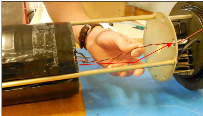
*Figure C.2-4: Align Battery to Fit Connector Through Hole in Top Plate*
