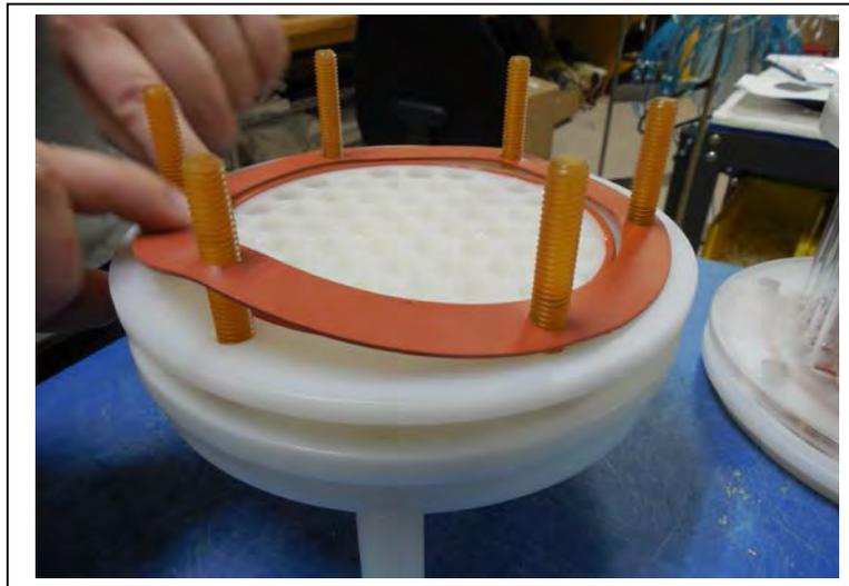
*Figure 6.2-7: Installing the Optional Gasket to Seal the Pre Filter*
