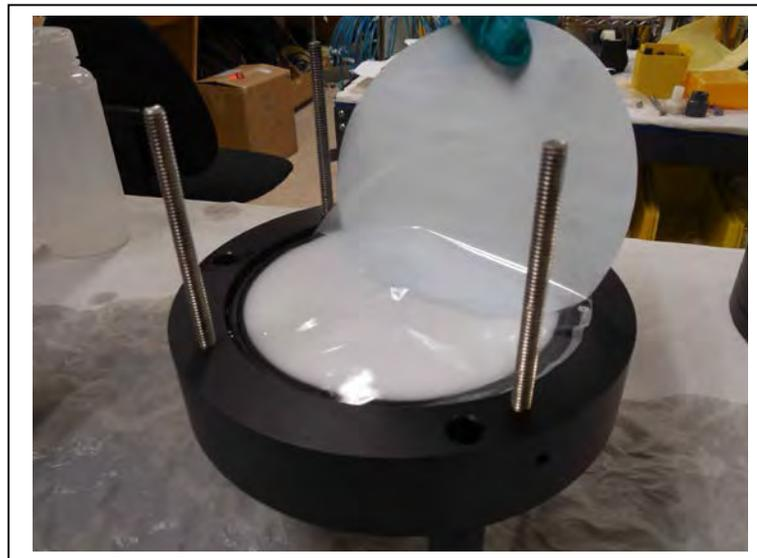
*Figure 6.1-3: Placing the Filter on the Bottom Filter Holder Plate*
