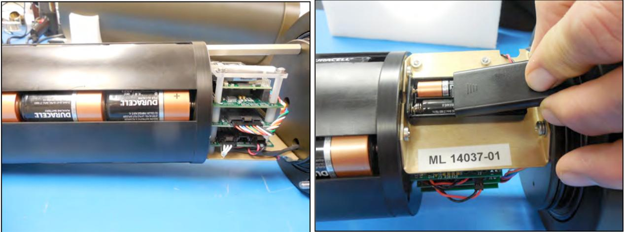
*Figure C.3-13: Main and Backup Batteries*
