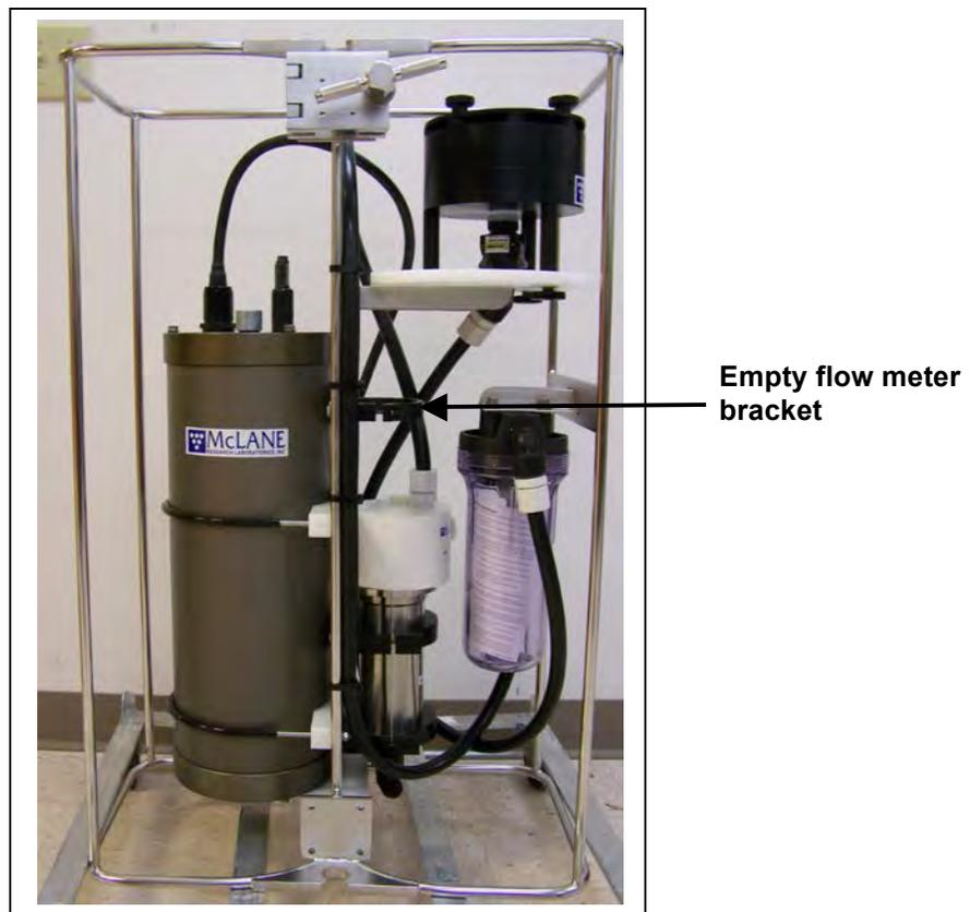
*Figure F-1: WTS-LV Upright with 30L/min Pump Head*
