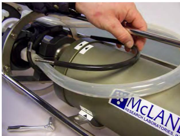
*Figure C.3-11: Removing U-Bolt*
