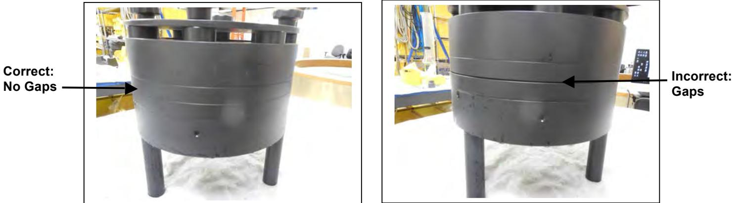
*Figure 6.1-10: Correctly Closed Filter Holder    Figure 6.1-11: Incorrectly Closed Filter Holder*
