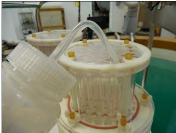
*Figure C.1.3-11: Filling Filter Holder Top with Water*
