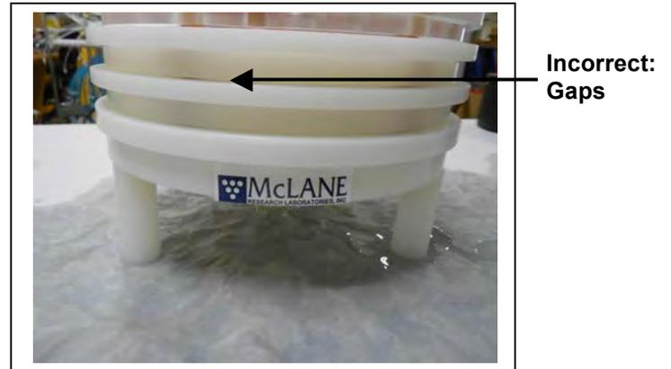
*Figure 6.2-10: Correctly Closed Filter Holder*    *Figure 6.2-11: Incorrectly Closed Filter Holder*
