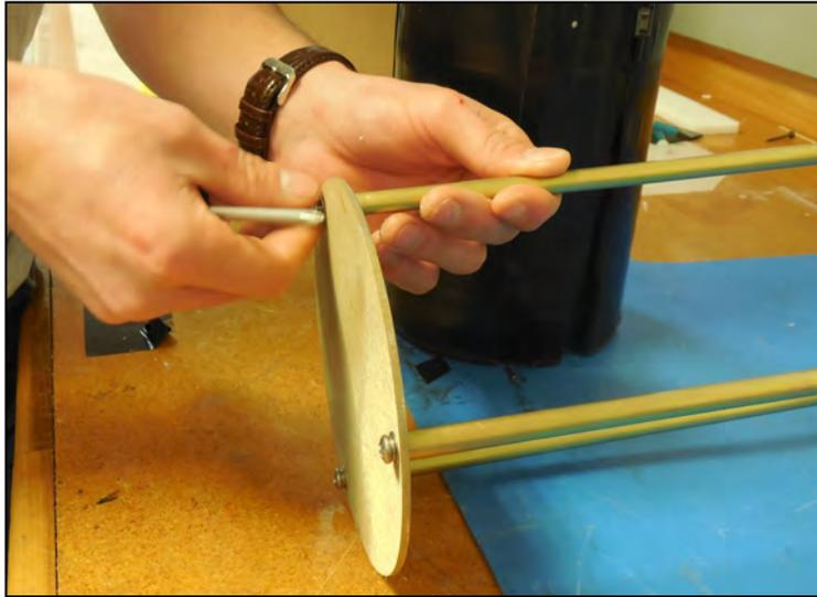
*Figure C.2-3: Removing Battery Housing End Plate*
