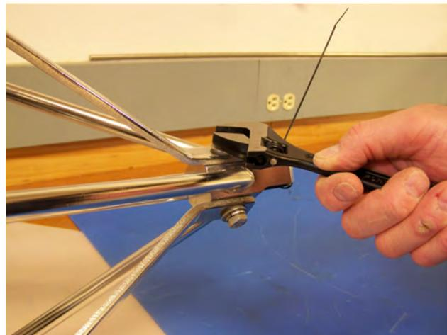
*Figure C.3-8: Loosening Frame Guard*
