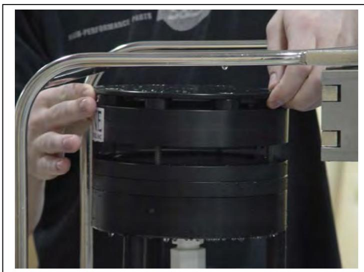
*Figure D-2: WTS-LV 3-Tier Filter Holder*
