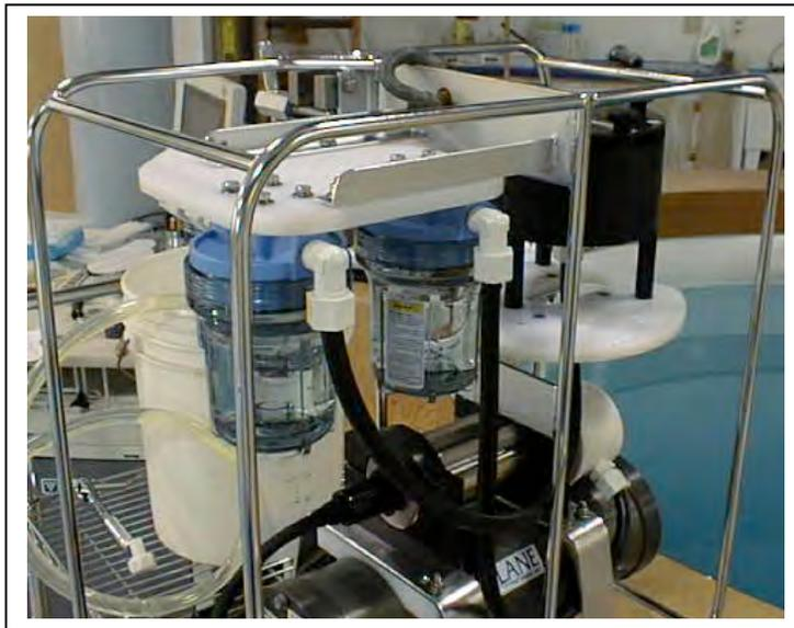
*Figure D-3: WTS-LV with Cartridge Filter Holders*
