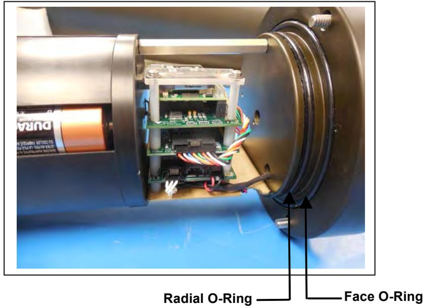
*Figure 4-5: Controller Housing Top End Cap, with O-Ring Seals*
