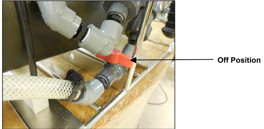
*Figure C.1.3-10: Setting the Flow Valve*
