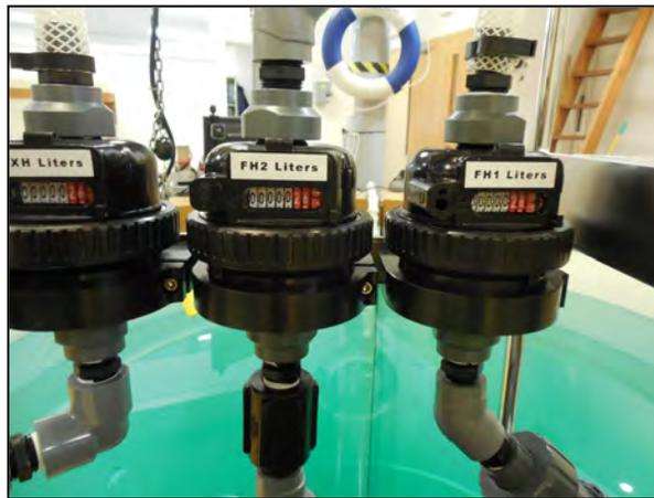
*Figure C.1.3-12: Mechanical Flow Meters*
