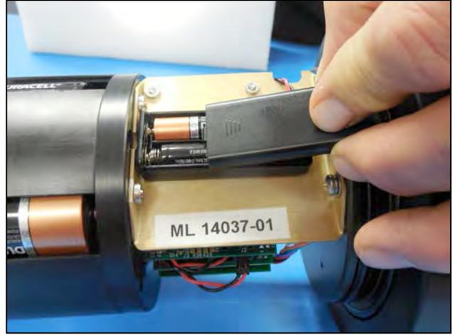
*Figure 5-6: Backup Batteries*
