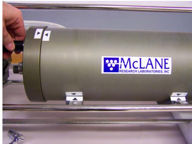
*Figure C.3-14: Returning Controller to Frame    Figure C.3-15: Aligning Arrows, Reattaching Connector*
