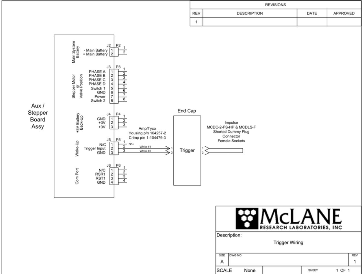
Figure 5-7: WTS-LV Trigger Wiring
