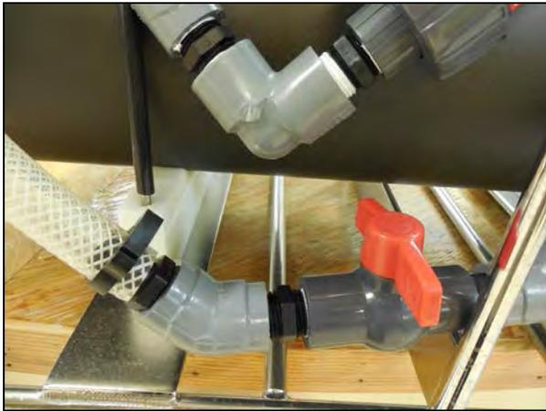
*Figure C.1.2-1: Valve Closed*
