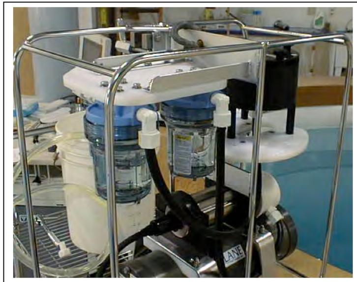
*Figure D-3: WTS-LV with Cartridge Filter Holders*
